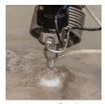
Automatic water Raise/Lower at the push of a button for Submerged Cutting; our tanks include air-tight welds of an air chamber which uses regular shop air pressure.
