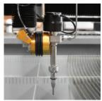
When the cutting head inadvertently crashes into a clamp or fixture, or hits the edge of a work piece or an upturned part, the Break Away Head will detect the crash and automatically stop the machine.
