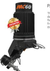
The PAC 60™ operating software incorporates the True Cut® algorithms data base, developed to determine the predicted taper at a given surface finish. This taper is then compensated for when cutting the part, anywhere from 0 to 60 degrees, giving you "Precision Angle Control" of any part that can be produced on an X-Y abrasive waterjet cutting machine.
