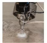
Automatic water Raise/Lower at the push of a button for Submerged Cutting; our tanks include air-tight welds of an air chamber which uses regular shop air pressure.
