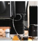
Programmable Z axis with auto height position recall, laser terrain mapping and edge location optics.
