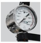
The HP gauge displays the pressure on the high-pressure water line. This allows the operator to see the actual pressure supplied to the cutting head and assists in troubleshooting.
