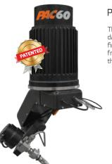
The PAC 60™ operating software incorporates the True Cut® algorithms data base, developed to determine the predicted taper at a given surface finish. This taper is then compensated for when cutting the part, anywhere from 0 to 60 degrees, giving you "Precision Angle Control" of any part that can be produced on an X-Y abrasive waterjet cutting machine.
